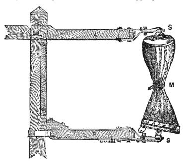
but most of it in the bottom. Buckle the strap around the center of pouch M. In case the strap is gone, tie the middle of the pouch, as seen in the diagram. It is worse than useless to hang up a bag crammed full like a bag of grain.
